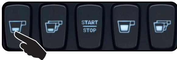
During this phase, the value of the pulses of the volumetric dispensing device (at the top right of the display) increases. On releasing the button, the value reached is stored and appears under the key programmed.
