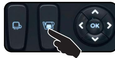
During this phase, the time in seconds (at the top right of the display) increases. On releasing the button, the value reached is stored and appears under the key programmed.
